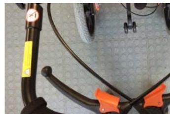
**Note:** Check the catch-mechanism and secure with locking pin after attaching seat!
