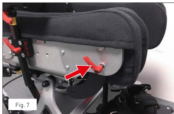
seat shell (Fig. 7) counterclockwise until the foot rest can be moved. Make sure not to turn the clamp lever more than necessary, otherwise there is a risk of the lever popping out of the thread. To deactivate the foot rest mechanism, turn the clamp lever clockwise until the foot rest is firmly locked again.
